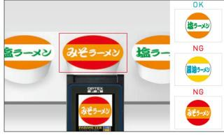
**CVS2-RA** Check the color and shape by its pattern matching function
